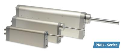
Motor series with independently programmable linear and rotary direct drives in a slim housing. Available with the following optional features: built-in precision torque measuring, integrated force sensor, vertical load compensation and hollow shaft. A complete stainless steel version is also available on request.
