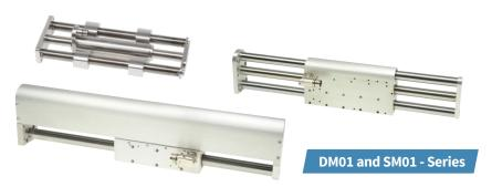
Linear modules with protection class IP64S and stainless steel linear modules with protection class IP69 consisting of a linear guide and an integrated LinMot linear motor. Optionally equipped with the MagSpring® magnetic spring and a pneumatic holding brake. The motors offer stroke lengths up to 680 mm and a peak force up to 572 N.
