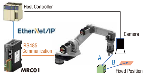
Figure 15. Cooperation between Robot and Camera
