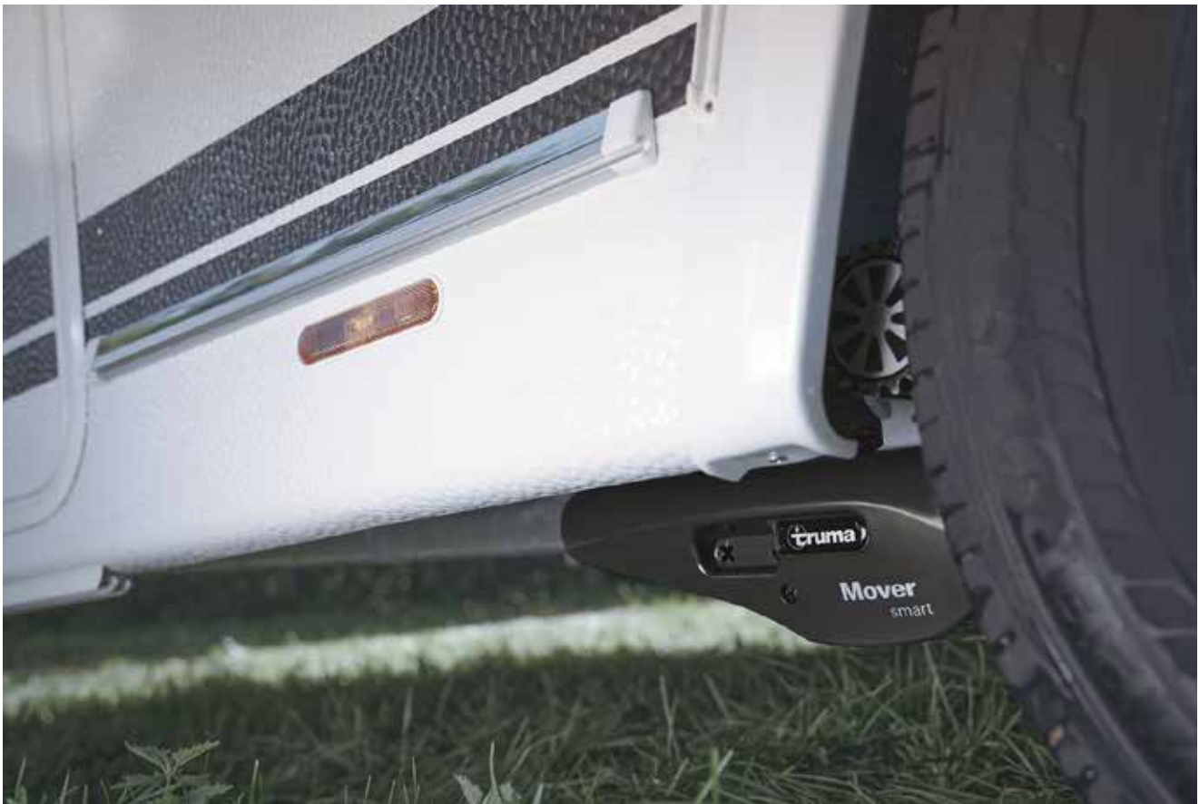
The Smart Mover is the heart of the system – powered by Parvalux motors.
